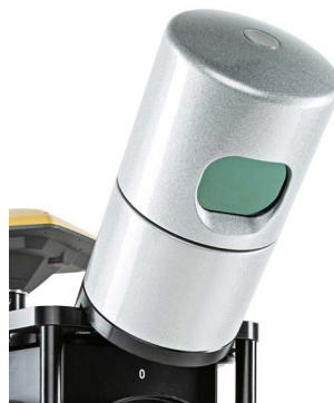
32 lasers, calibrated by Topcon
