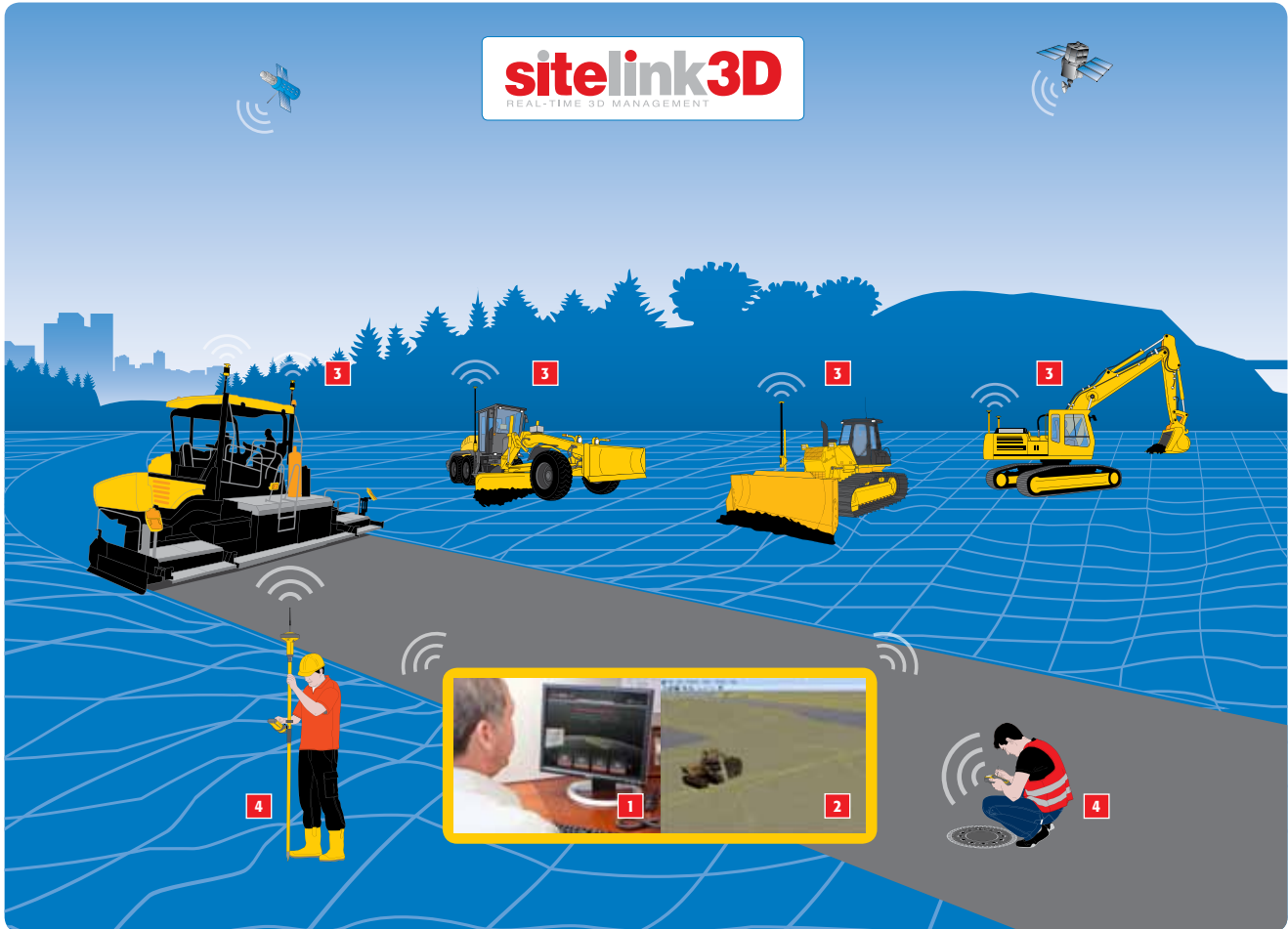
1 Web Portal Access 2 Sitelink 3D Interface 3 Machines 4 Surveyors
